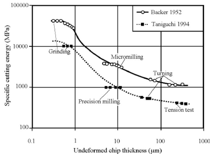
**Figure 1:** Variation in specific cutting energy for three major machining processes [16].
