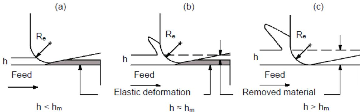
**Figure 3:** Schematic diagram of the effect of the minimum chip thickness [15, 18]
