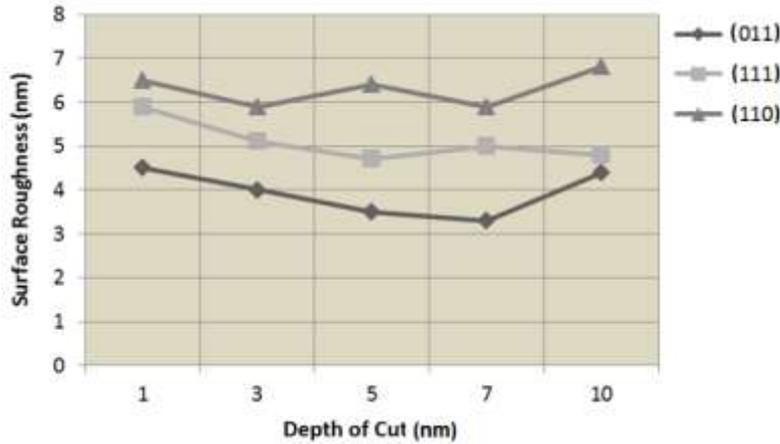
**Figure 2:** Effects of the crystallographic orientation and the depth of cut on the surface roughness conducted by the diamond turning of single-crystal aluminium rods [15].
